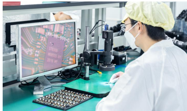
Microscopic inspection: 20X
