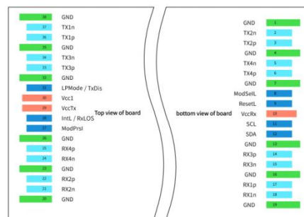
Figure4:QSFP112 Module contact assignment
