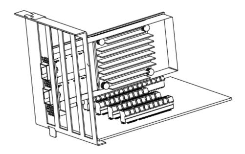
6. Secure the adapter with the adapter clip or screw.
