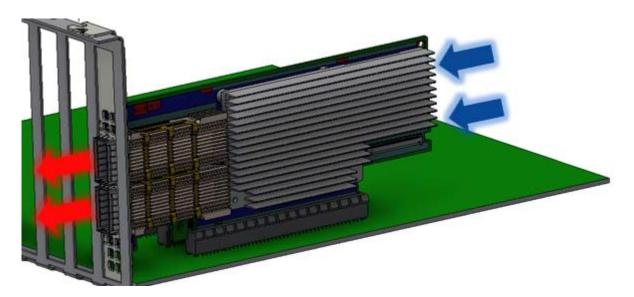
Airflow *from the network ports* to the heatsink:
