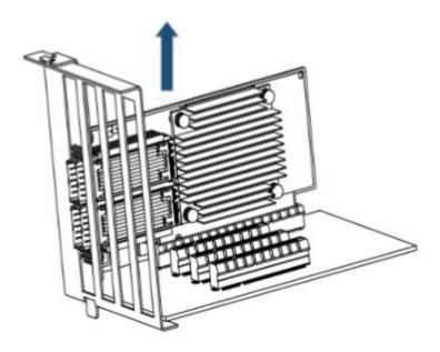
5. When the port connectors reach the top of the chassis window, gently pull the adapter card in parallel to the motherboard.
