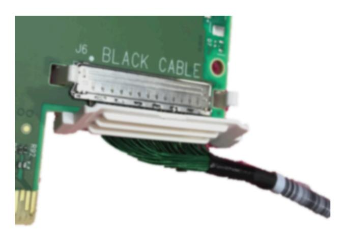
**Step 4:** Clamp the retention clip. Verify both latches are firmly locked.
