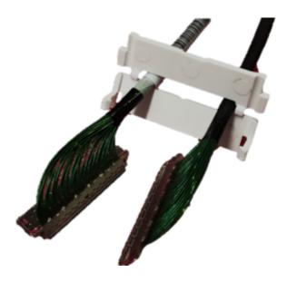
**Step 6:** Plug the Cabline CA-II Plus harnesses into the PCIe Auxiliary Card. As indicated on both sides of the Auxiliary connection card, plug the black harness into the component side and the white harness into the print side.
