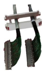
**Step 2:** Plug the Cabline CA-II Plus harnesses into the ConnectX-7 adapter card while paying attention to the color coding. As indicated on both sides of the card, plug the black harness into the component side and the white harness into the print side.
