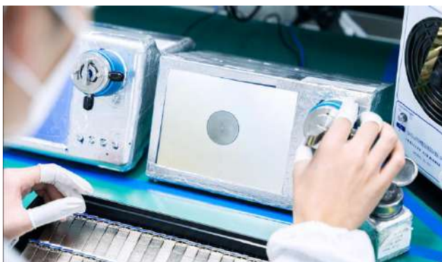
Optical endface inspection
