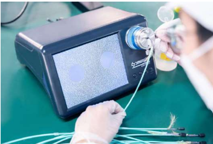
End Face Inspection
