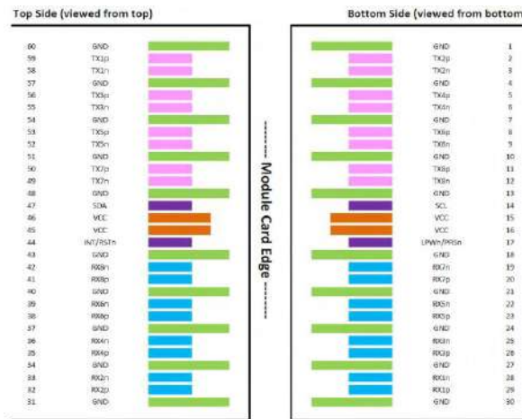
Figure3:OSFP Pin view
