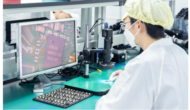
Microscopic inspection: 20X
