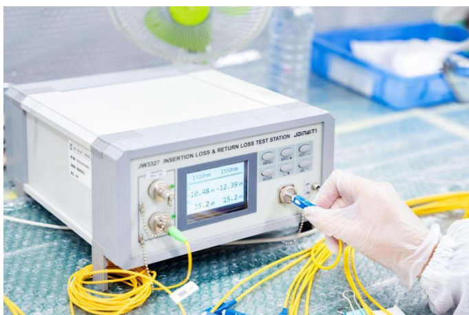
Insertion/Return Loss Test
